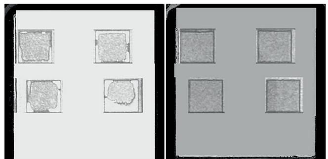
**Figure 3:** On the left we have a SAM image of dies showing varying degrees of delamination. Deep power cycling (which equates to thermal cycling) will cause further delamination. On the right we have a SAM image of good sintering results
