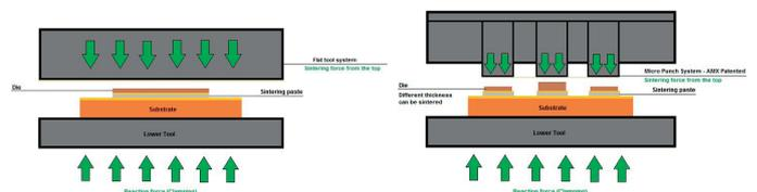
**Figure 2:** Above, on the left, a standard flat, single punch sinter tool. Ideal if you are sintering a large, single die. Dies are getting smaller though and power modules are likely to have several dies with different thicknesses. The micro-punch system on the right applies equal force to all dies.
