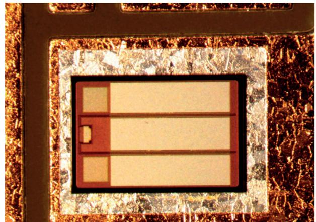
**Figure 1:** Above, a sintered SiC die. Image courtesy of AMX Automatrix.
